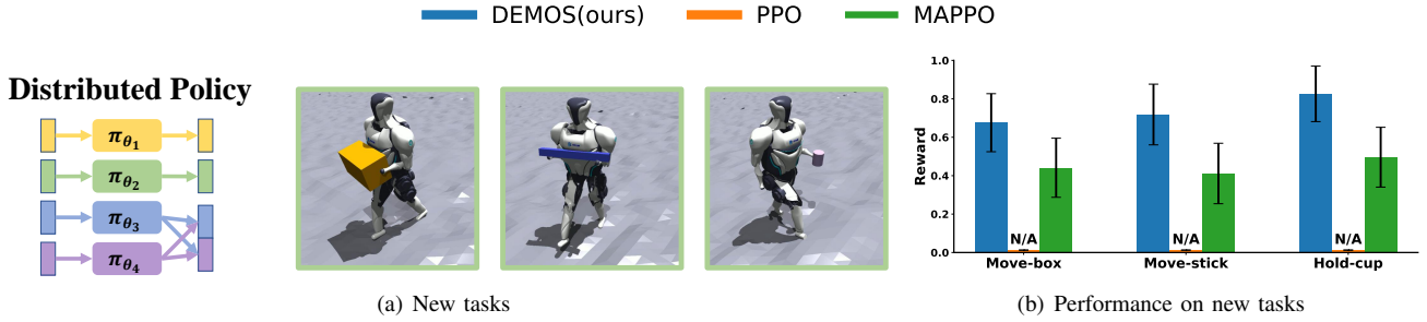
Fig. 7: Transfer part of the decentralized policy to new tasks: move-box task, move-stick task, hold-cup task.
